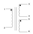
Primary: Secondary: 1 to 2 Series - 3 to 6, Jumper 4 to 5 Parallel - 3 to 6, Jumper 3 to 5 and 4 to 6
